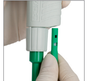
Adjustable ejector height system – to accommodate various brands of tips
